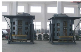
10吨钢壳炉体 10 tons steel shell furnace
