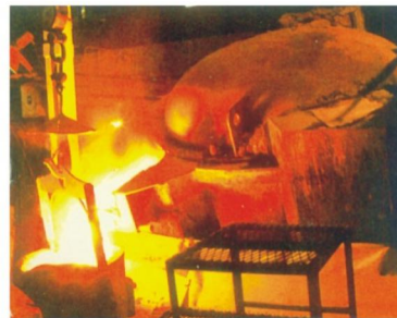
3吨工频有芯熔铜炉 3 tons power frequency induction furnace for melting copper
