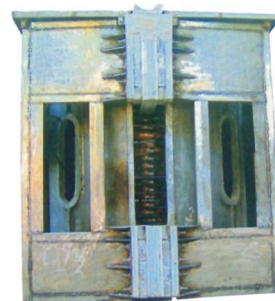
10吨铝芯不锈钢壳中频熔炼炉 10 tons stainless steel shell IF melting furnace
