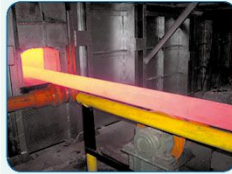
钢管淬火 Steel tube quenching
