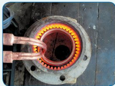
齿轮内齿淬火加热 Gear inner teeth heating for quenching
