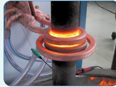
小轴淬火 Small shaft quenching
