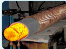
工件在线加热 Workpiece online heating
