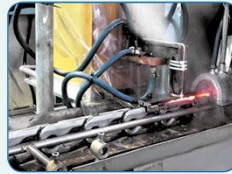
履带轨节淬火 Track joint quenching
