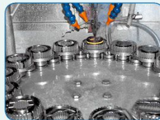
异形齿轮内孔淬火 Inner hole quenching of special gear
