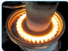
花键轴淬火加热 Spline shaft heating for quenching
