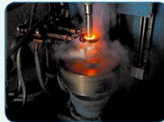
引导轮表面淬火 Guide wheel surface hardening
